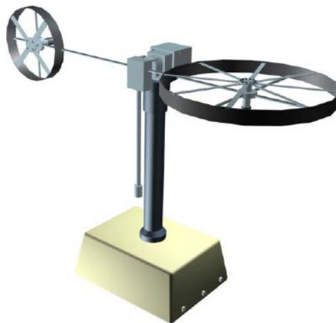
Figure 1: TRMS Mechanical Unit
